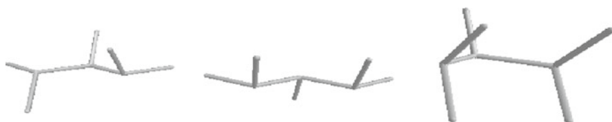
Fig. 4 Dualists of 3 octamantane valence isomers, namely a regular [1(2)3(2)1(3)4]octamantane and two irregular octamantanes: [1(2)3(2)1(2)1]octamantane having one proximity, and [1(2)3(1)4(1)2]octamantane with two proximities
